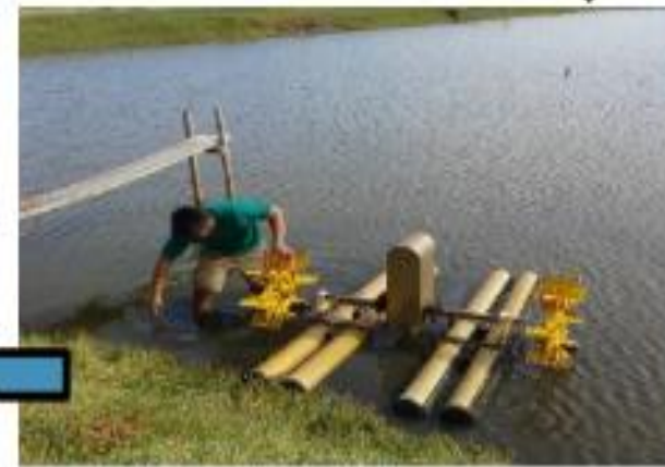
5. Provision of life support systems: paddle wheel and water pumps
